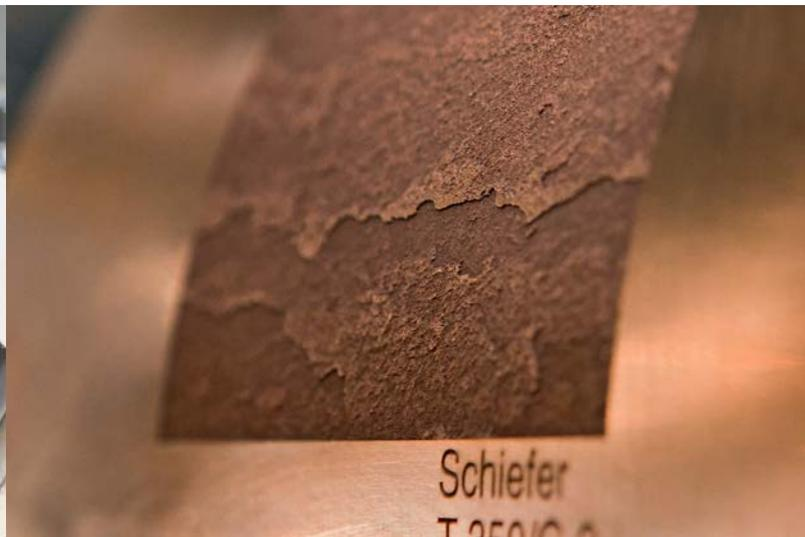
**Exciting surfaces through 3D embossing.** Within the framework of various research and development projects, we use the latest laser technologies and are continually expanding their range of applications. Here, the field of embossing in particular offers very exciting possibilities. In addition to the traditional engraving in copper, we are also experimenting with alternative surface materials and are optimising the use of three-dimensional embossing structures.
