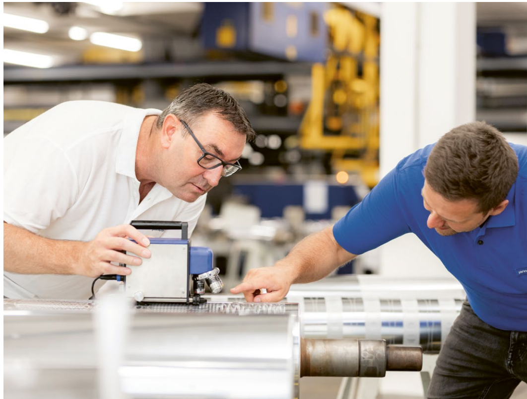
The experts use a 3-D microscope to check whether the cylinder has been produced in line with specifications. The microscope measures the geometry and volume of the cells.
