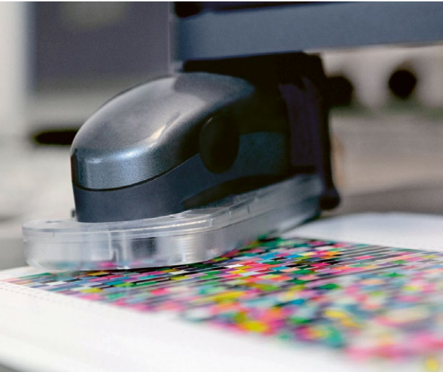
Meticulous measurement of the whole print sheet: a measuring instrument runs over each of these charts, known as "GMG ECI 2002 random", using the 1,504 different coloured measuring fields to create a profile.
